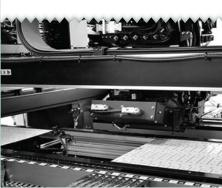
LED components are mounted on the board through automation. Specially designed electronic circuits and LED components are placed onto the boards which are reinforced with a high density aluminium base.
