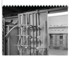
**Electrostatic-lamination painting is carried out.** Electrostatic powder paint is a completely dry coating method which does not contain any solvent. Powder paint is applied using special painting pistols in a paint booth.
